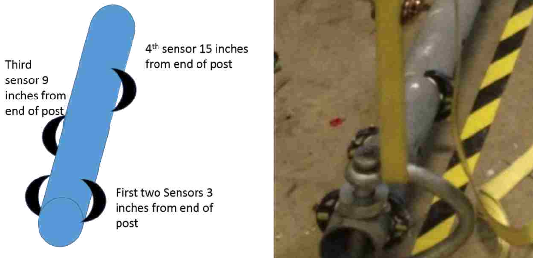
Figure 31. Illustration and photograph of seaweed sensor placement for the first post installation
