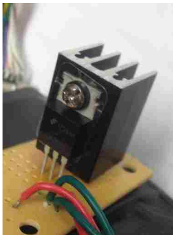
Figure 26. Heat sink used to prevent overheating of the 5V regulators
