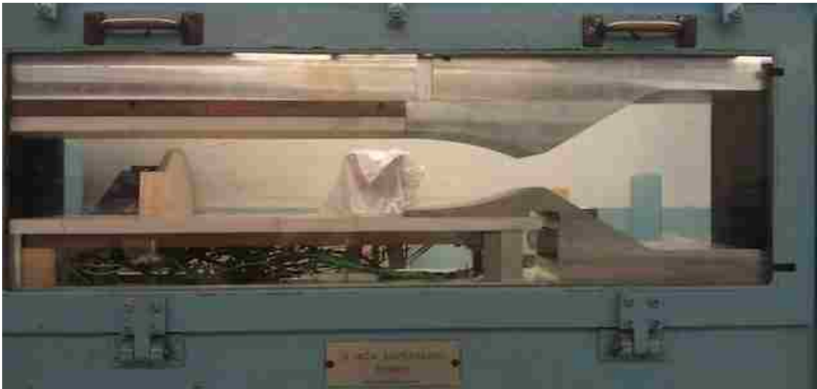
Figure 3.3: Full experiment installed in wind tunnel. Nozzle blocks can be seen on the right side of the test section feeding into the instrumented MACOR ® surfaces in the center. These surfaces are attached to the copper heating plates.
