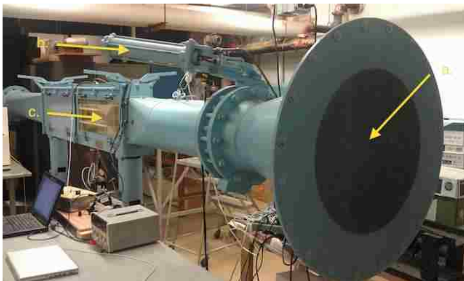
Figure 3.1: University of Maryland supersonic wind tunnel. In near field right, the intake bell (a.) can be seen. In the center of the picture, the butterfly valve and control arm are shown (b.). At the far left is the test section housing the experiment and instrumentation (c.).
