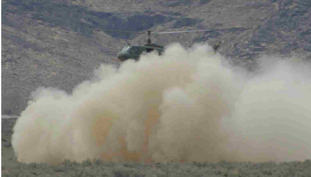
Figure 1.1: Rotor-induced sediment mobilization, or “brownout” (Courtesy of Optical Air Data Systems LLC.)
