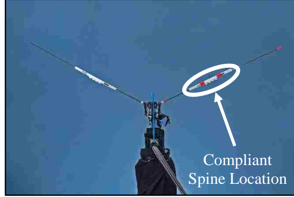
Figure 35. Example of a leading edge spar-spine configuration that was used to validate the leading edge spar analytical model.
