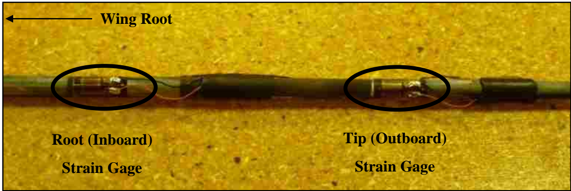
Figure 25. Strain gages mounted on the leading edge spar at the location of the compliant spine root and tip
