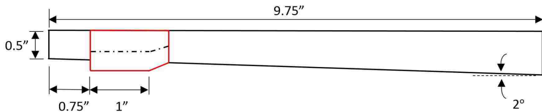
Figure 5.10: Thermally choked cavity combustor with heat release domain broken into 2 equal parts by the centerline. Each part will be modeled separately with equal heat release densities and compared.
