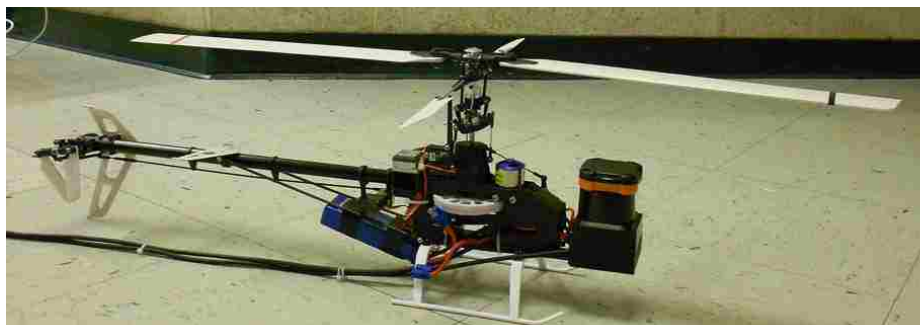
Figure 4.6: Blade 450 helicopter. Laser scanner mounted at the front.
