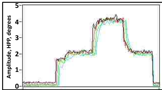
Figure 4.3: All 4 Flaps on Two Blades Amplitude Closed-Loop Control at 900 RPM
