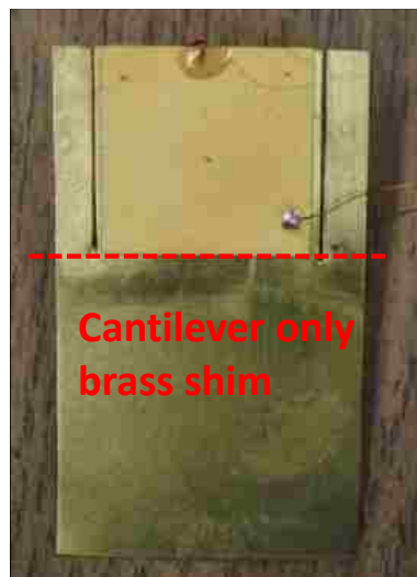
Figure 2.35: PZT-5K4 Bimorph with No Piezoceramic in Cantilever ('Dead')
