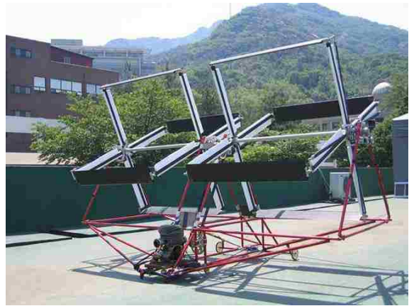
(b) 43 kg twin-cyclocopter UAV.
