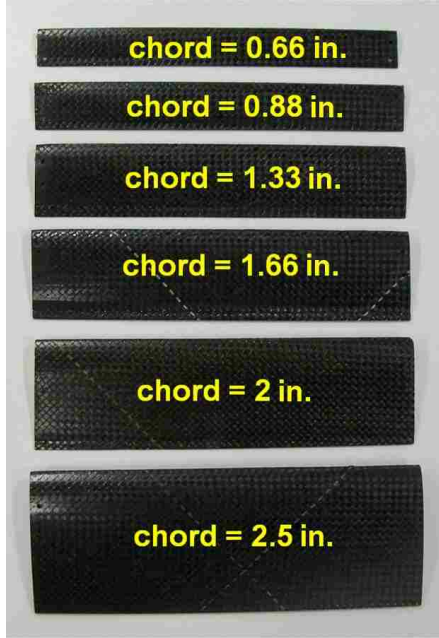
Figure 5.1: Blade chord lengths tested to vary c/R ratio.
