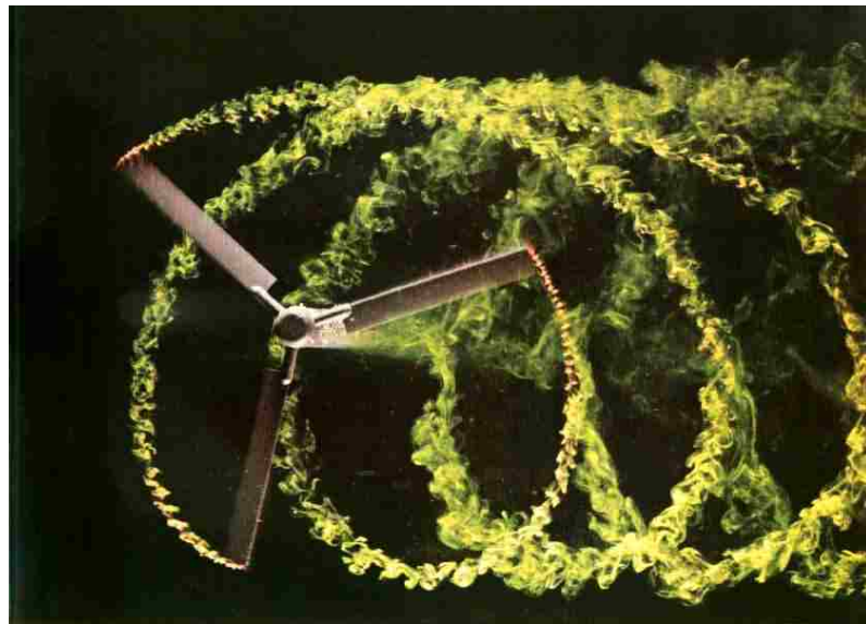
Figure 1.5: Visualization of Tip Vortices - Ref. [28]
