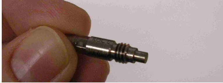
Figure 4.14: Photograph of the uninstalled PCB 105C12 dynamic pressure sensor.
