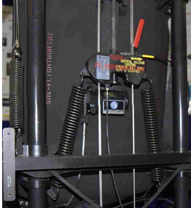
Figure 21: Seat Bracket Clearance when Raising Crossbar
