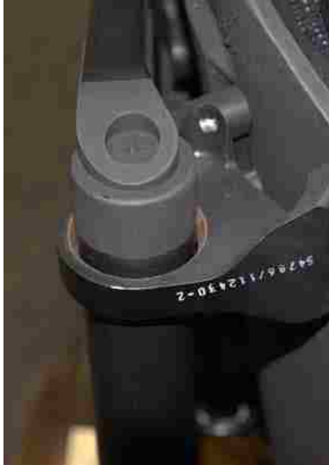
Figure 22: Loosely Fitted Guide Tube Bearings
