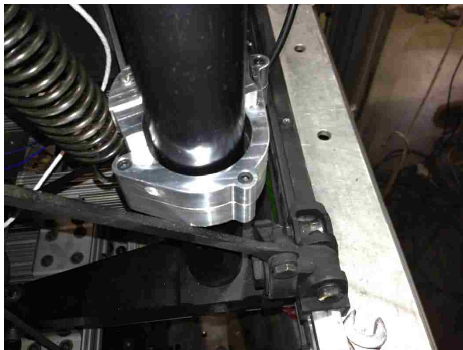
Figure 106: Lower Bracket - Right Side (From the back) - X-bar Clearance Issue
