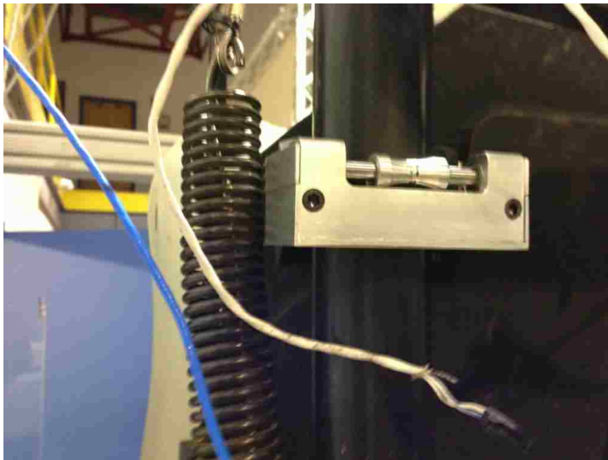
Figure 102: Upper Bracket - Armor Side - Spring Clearance Issue on Crash Stroke
