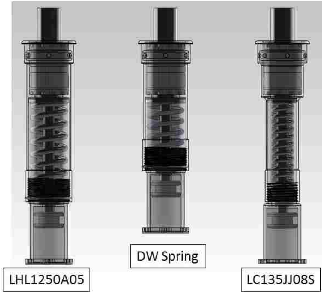
Figure 41: Effect of Spring Options on Damper Integration Design
