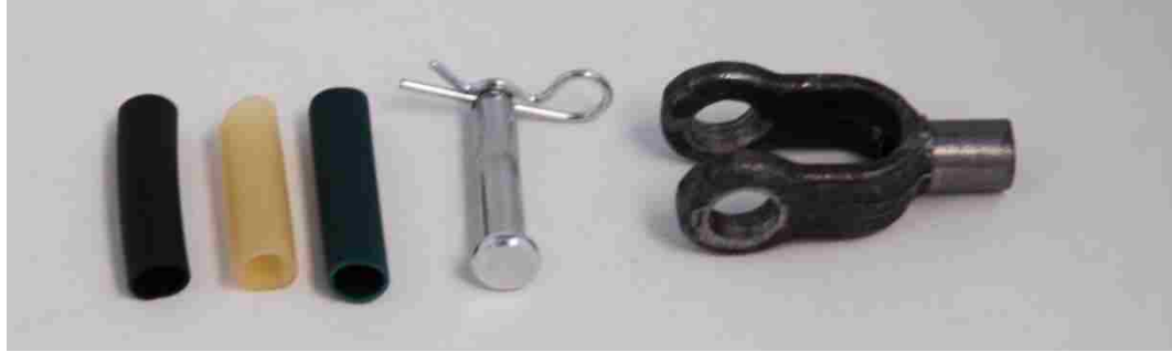
Figure 144: Large Clearance Clevis and Samples of Tubing from Testing
