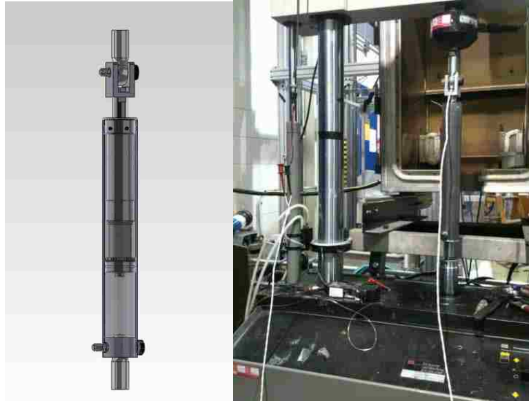
Figure 48: MTS Mounting Design CAD Model and set in MTS Machine
