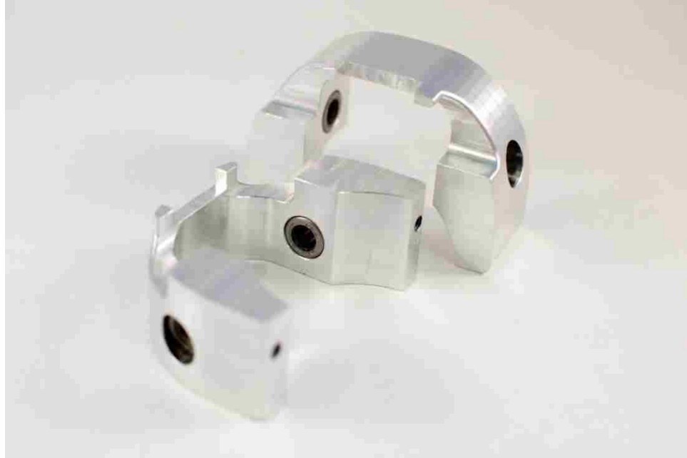
Figure 89: Lower Assembly - Bearing Holders
