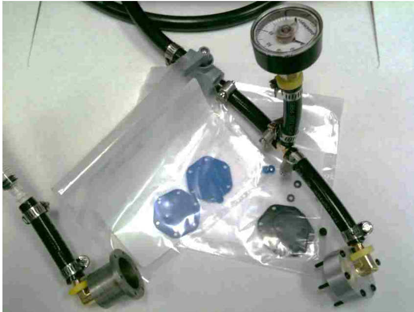
Figure 43: Diaphragm Test Setup
