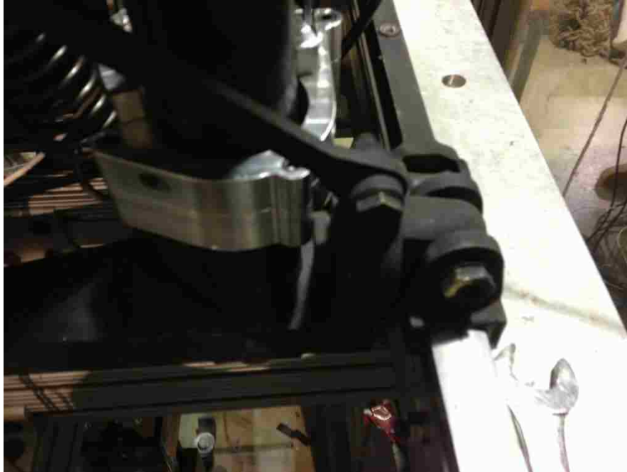
Figure 107: Lower Brackets Clearance on Full Down During Crash Stroke
