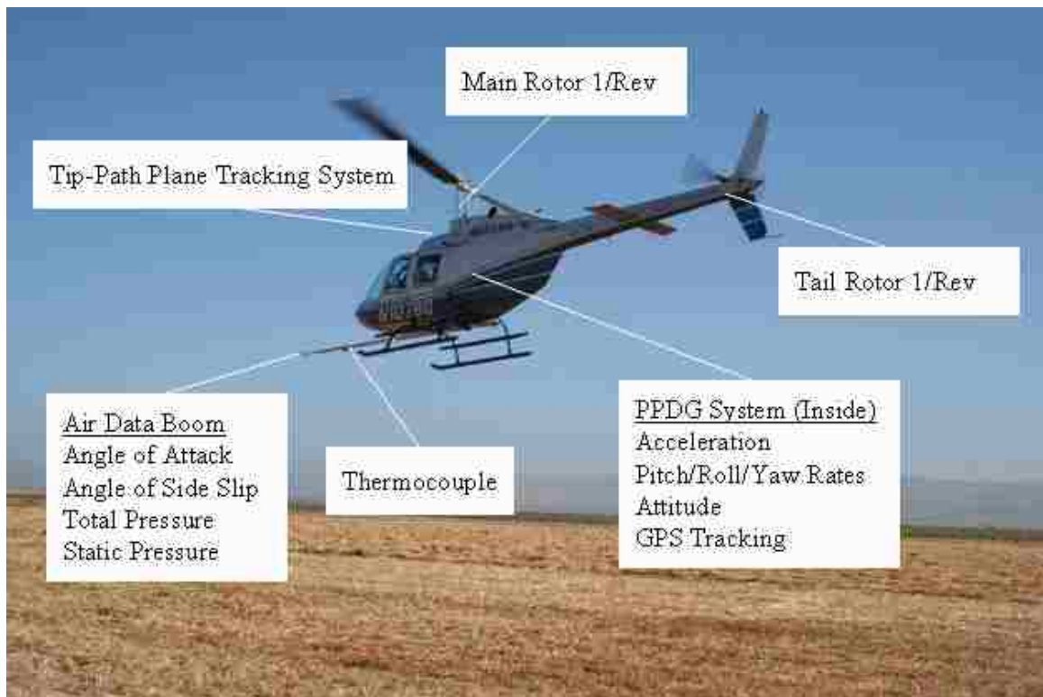
Figure 2.3. Bell 206B-3 in-flight instrumentation package.
