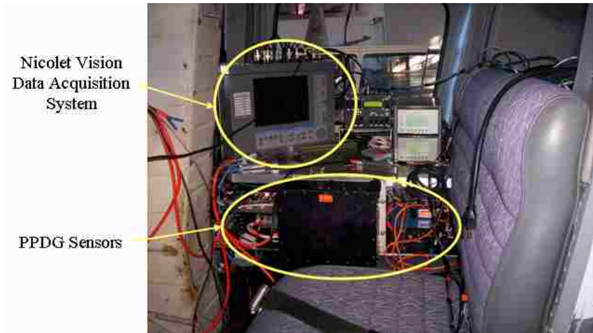
Figure 2.4. In-flight measurement pallet.
