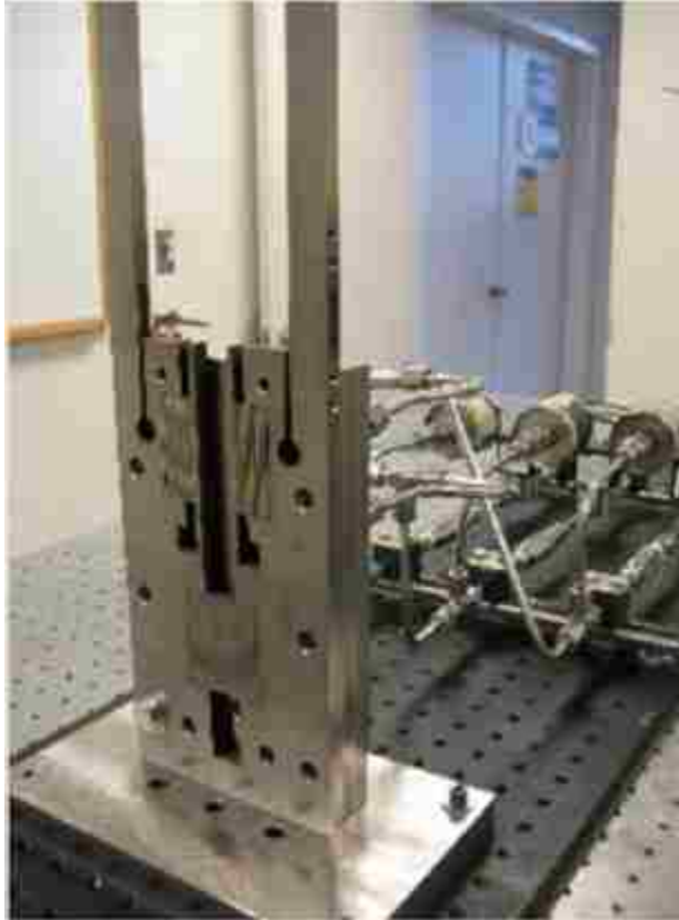
Fig. 3.6 Picture showing cutaway of combustor inlets (Ghosh, 2008)
