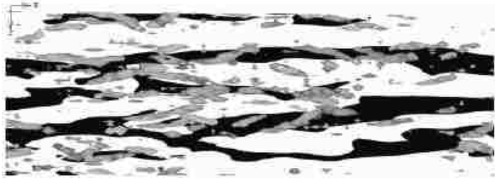
Figure 2. 7 Near-wall structures comprising lifted low-speed streaks (black) and quasi-streamwise vortices (grey). Images adopted from [42].
