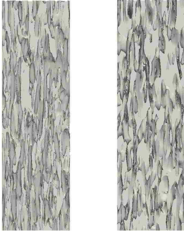
Figure 5. 37 Instantaneous isosurface of the second invariant of the velocity gradient tensor, Q > 0 , (left) RLES \Delta y_{\text{wall}} = 1 mm, (right) ErfWF \Delta y_{\text{wall}} = 5 mm at y^x \approx 10 .
