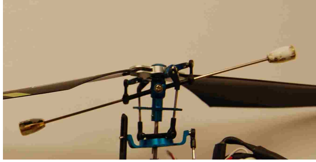
Figure 1.3: Flybars are used to mechanically stabilize helicopters.
