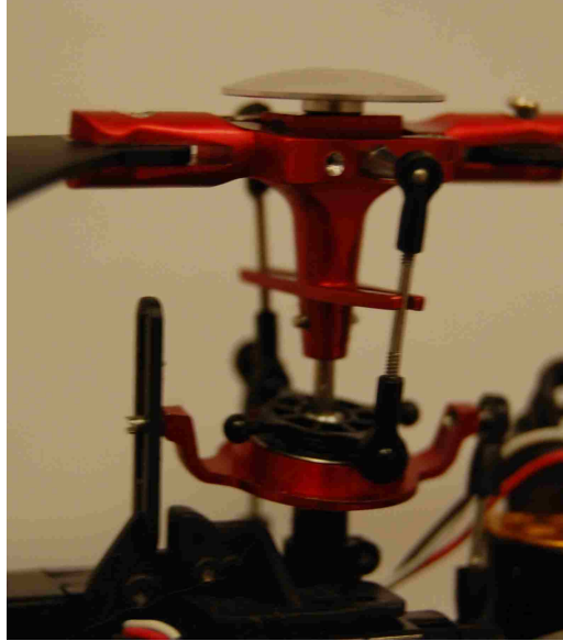
Figure 2.4: The servos tilt the swashplate which, through mechanical arms, pitches the rotor blades.
