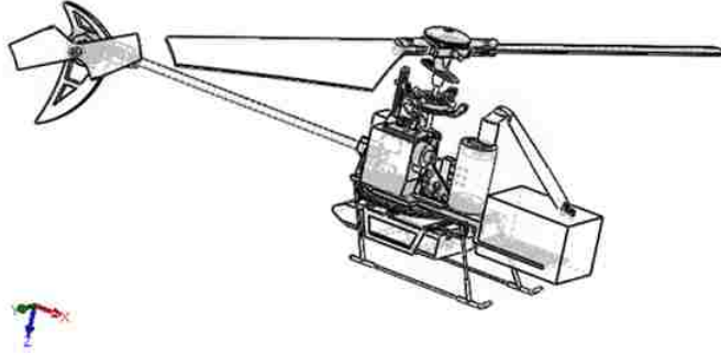
Figure 1.2: A SolidWorks model was used to calculate the moments of inertia of the helicopters. (CAD credit: Julia Ashkanazy)
