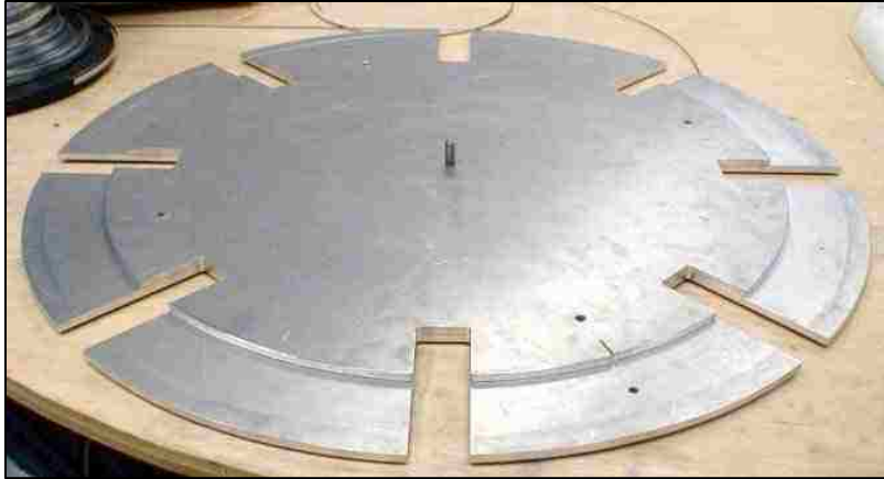
Figure 7 – Spool Used to Manufacturer Coil Layers
