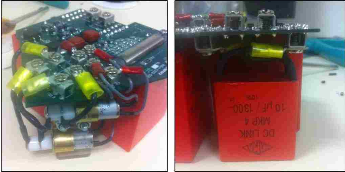
Figure 62 – Wire Connections from Capacitor Board to Relays and WPT Capacitor
