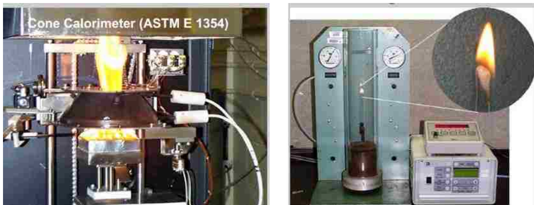
Figure 1-5. Bench apparatuses adopted from Ref. [4, 6]: Cone calorimeter (left), and oxygen index (right)
