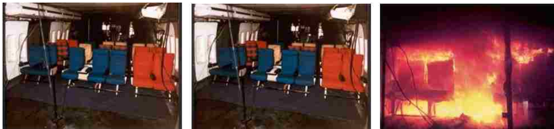
Figure 1-7. Full scale cabin mock up: development of Fire Test for Aircraft Seat Cushion [11]
