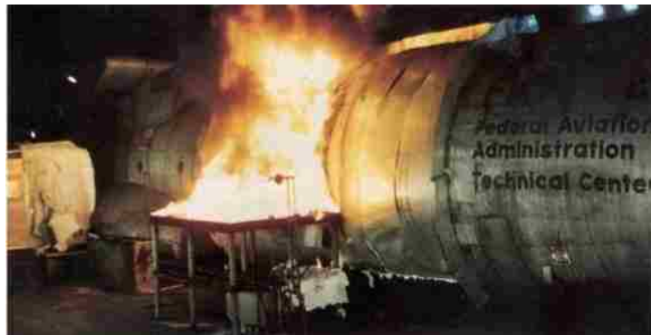
Figure 1-6. Post-crash fire simulation in a full-scale indoor fire test facility [11]
