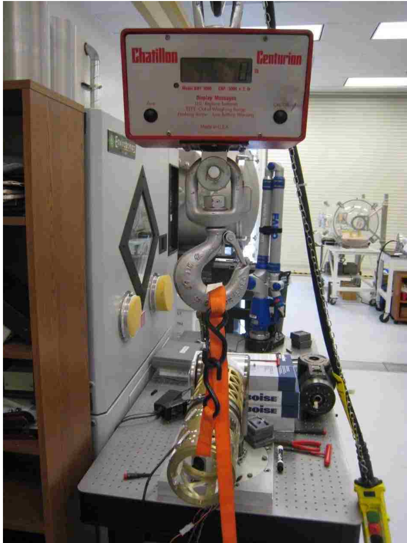
Figure 26 – Crane Scale Test Setup for Current/Torque Test
