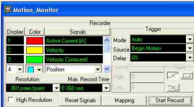
Figure 20 – Elmo Composer Motion Monitor Control Panel
