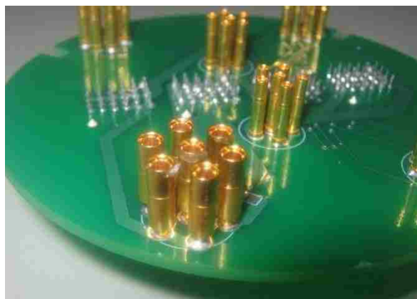
Figure 18 - SAMURAI Penetrator Board with Hypertronics Penetrator Pins
