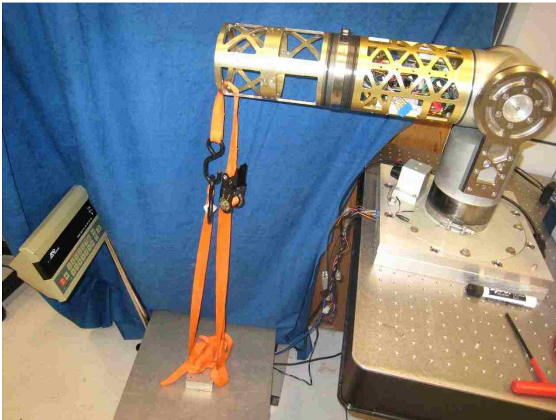
Figure 25 - Electronic Balance Test Setup for Current/Torque Tests
