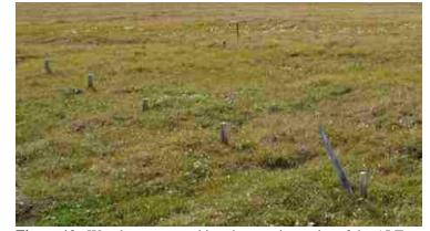
**Figure 10.** Wooden posts marking the exterior nodes of the ALT sampling grid at CRREL Plot 44 (Photo: Nikolay Shiklomanov).
