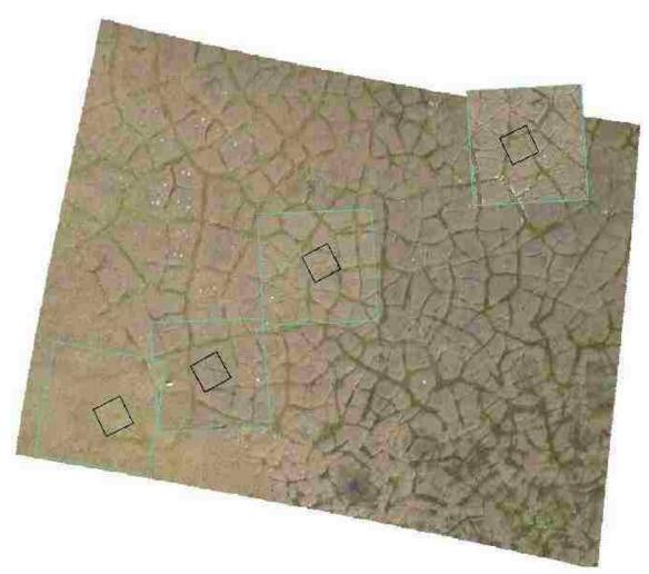
**Figure 12.** Georeferenced high-resolution kite photograph of the entire study area, overlain with cropped and independently georeferenced images of the individual study plots.
