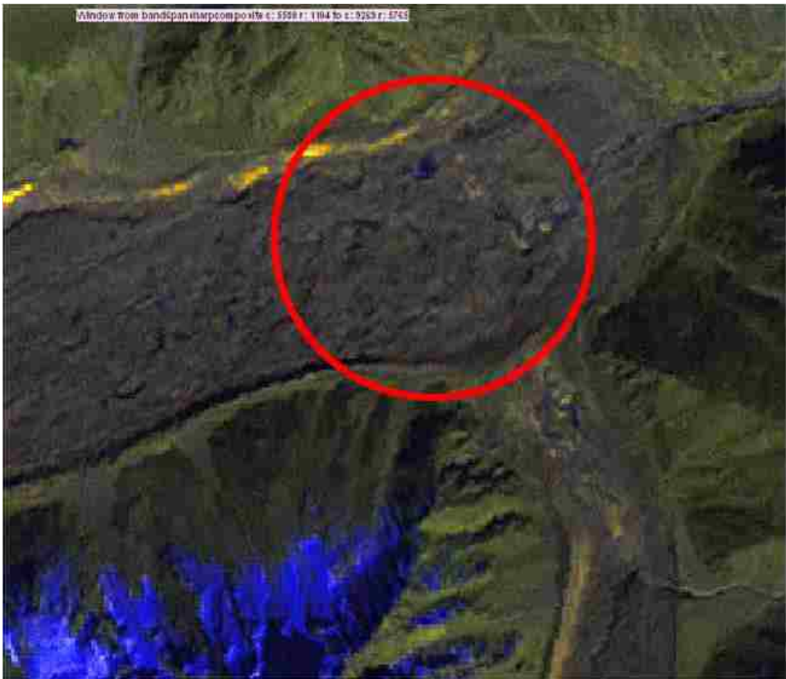
Figure 29. Landsat 7-5-1 image of a debris-covered glacier tongue in northern Pakistan. Note that the margins are indiscernible and do not differ in spectral signature from the glacier forefield.
