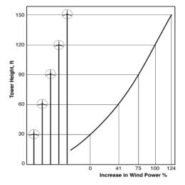
Figure 5. Theoretical Power Production for Small Wind Turbines When the Wind Speed is 10 m/s (DOE).
