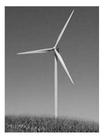
Figure 1. Horizontal Axis Wind Turbine (HAWT).
