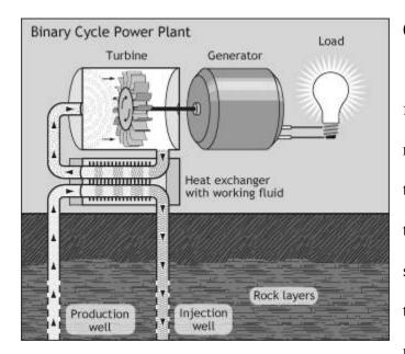
Figure 10. Binary Cycle Power Plant (Alternative Forms of Energy).
