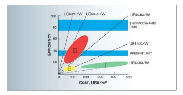
Figure 4. Efficiency and Cost Projections for First, Second, and Third-Generation PV Technology (School of PV and Renewable Energy Engineering).
