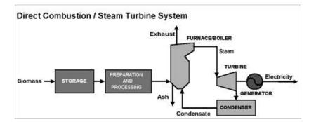
Figure 9. Electricity Generation from Biomass Combustion System (EERE).
