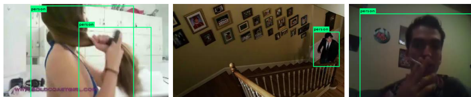
Fig. 4.9. Examples of human detection using YOLO algorithm from HMDB51 dataset. We can observe that YOLO fails to detect the person in the first image. It successfully performs human detection in the other two images.
