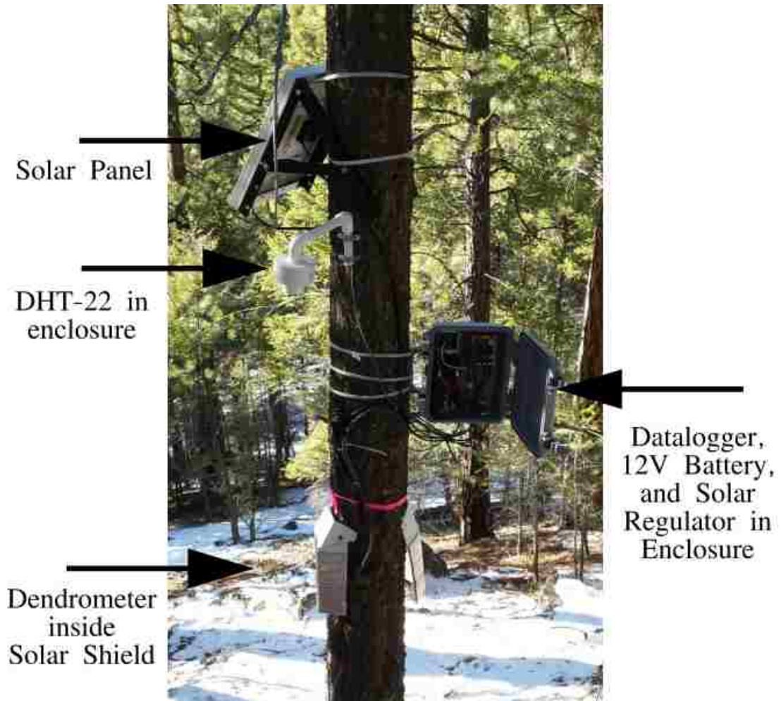
Figure 2.12: The Pinecone datalogger system fully installed on a tree in Lubrecht Experimental Forest. From top to bottom, a solar panel facing away from the camera, to recharge the system battery, A DHT-22 sensor inside a protective enclosure made from PVC piping, the opened case that holds the datalogger board, battery, and solar panel regulator, and shiny thermal protectors to shield the dendrometers from heating up in direct sunlight.
