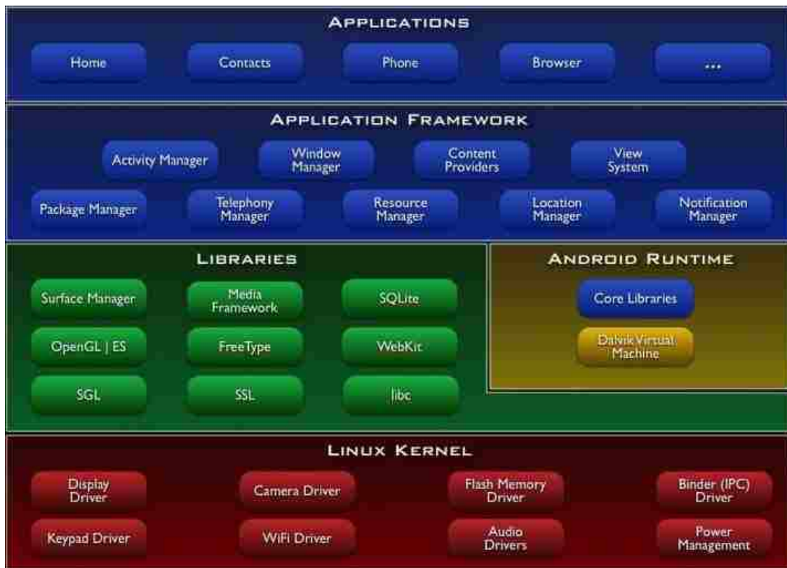
Figure 2: Architecture of the Android operating system.
