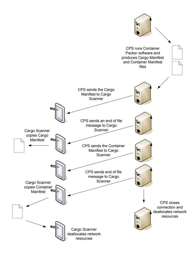
Figure 2.18 - Packing Process (Part 2)
