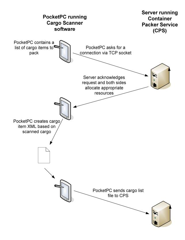
Figure 2.17 - Packing Process (Part 1)
