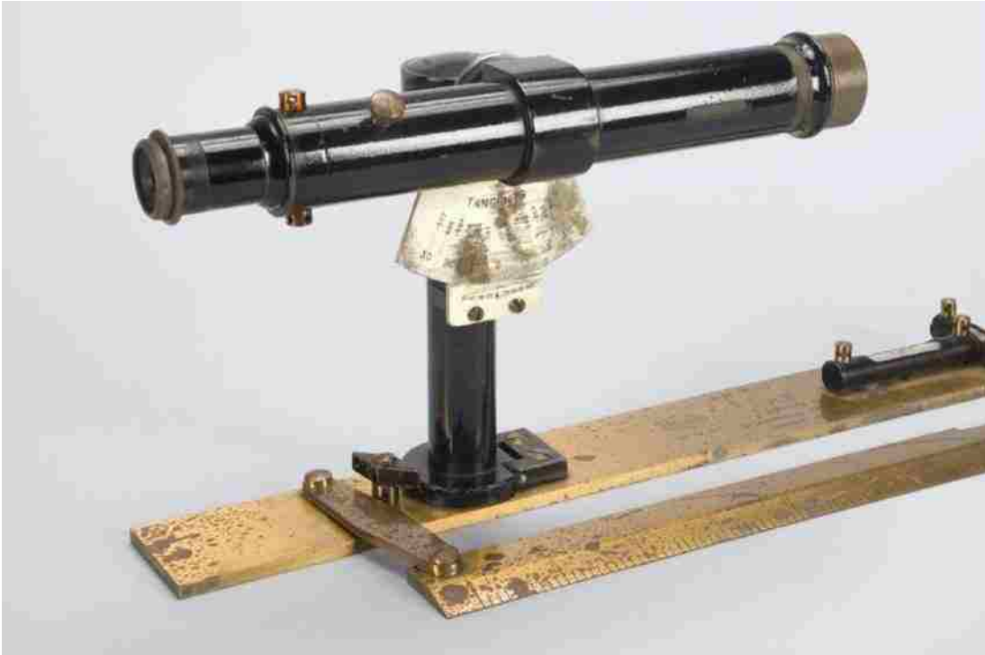
Figure 5. Telescopic distance finding alidade (Harvard).
