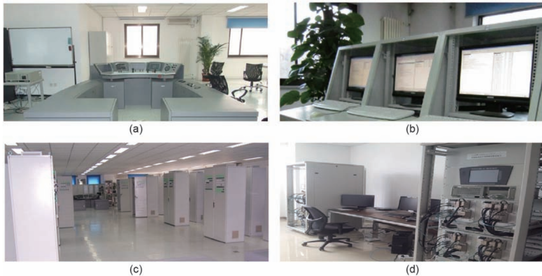
Fig. 4. The TCMS half-physical testing bench. (a) The driver control panel; (b) the simulation main control center; (c) the vehicle cabinets and the signal-processing cabinets; (d) HIL test.
