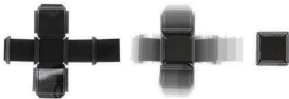
Fig. 5. Folding of an unpacked cube with hinges composed of a smart hydrophilic polymeric material; when submerged in water, the smart material actuates and the object folds into a cube. (Permission obtained from Ref. [16])
