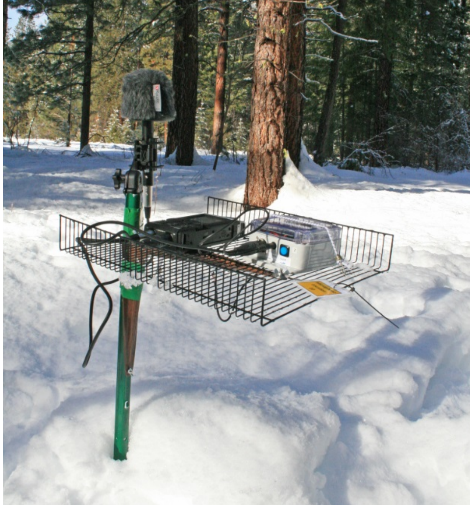
Figure 4: Microphone locations setup for each point on arrays. From left to right: Omni-directional microphone, solid-state digital recorder, and GPS clock synchronizer.
