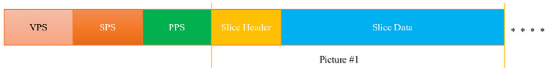
Fig. 4. HEVC bitstream NAL structure.
