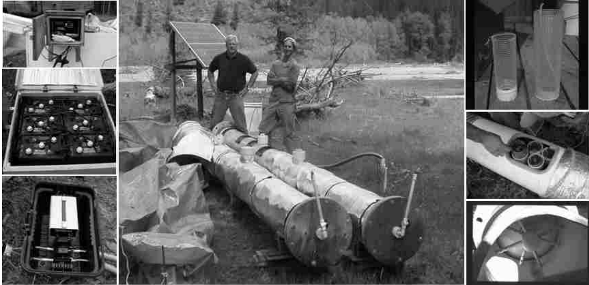
Figure 3: Close-up photos of hyporheic mesocosm components (counter-clockwise from upper left): solar controller, battery bank, peristaltic pump, inlet manifold (viewed through A1 access hatch, before gravel was introduced), sampling hatch with canisters, invertebrate sampling canister (l) and treatment canister (r). Center, paired mesocosms with authors for scale.
