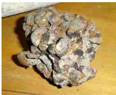
Figure 6: Treatment effect on experimentation canisters: (a) fine sediment only on the left, and sediment with organic matter on the right, the latter with a bullseye pattern of iron hydroxides (orange) and either manganese oxides or iron sulfides (black). (b) Coarse sediment ferricrete from the nearby Swan River aquifer, showing coarse grains with high pore space, cemented and coated with iron and manganese oxides.
