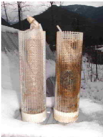
Figure 6: Treatment effect on experimentation canisters: (a) fine sediment only on the left, and sediment with organic matter on the right, the latter with a bullseye pattern of iron hydroxides (orange) and either manganese oxides or iron sulfides (black). (b) Coarse sediment ferricrete from the nearby Swan River aquifer, showing coarse grains with high pore space, cemented and coated with iron and manganese oxides.
