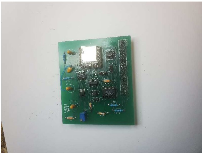
Figure 24 (above): The completed printed circuit card with mounted components.
