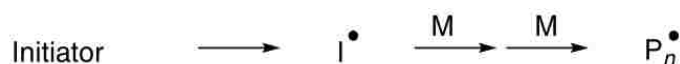
Figure 25 RAFT mechanism: Initiation. The initiator (I) is decomposed into radical ions (I • ) that react with monomer (M) and propagate to additional monomer to form polymer chains of n units (P n • ). The radical is conserved on the polymer chain as denoted by the dot (•). Reproduced from [167].
