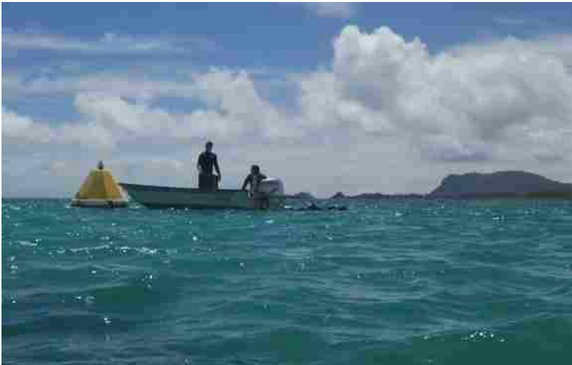
Figure 2:2 Divers at the CRIPM-2 buoy in Kaneohe Bay during the June 2013 SAMI-alk deployment. The MAPCO 2 system is housed inside the yellow buoy. The SAMI-alk was suspended below the buoy, see Figure 2.4.
