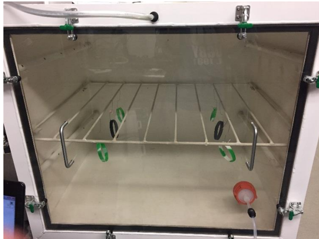
Figure 3: Close-up of exposure chamber, showing wristbands and the PTR-MS intake with filter.
