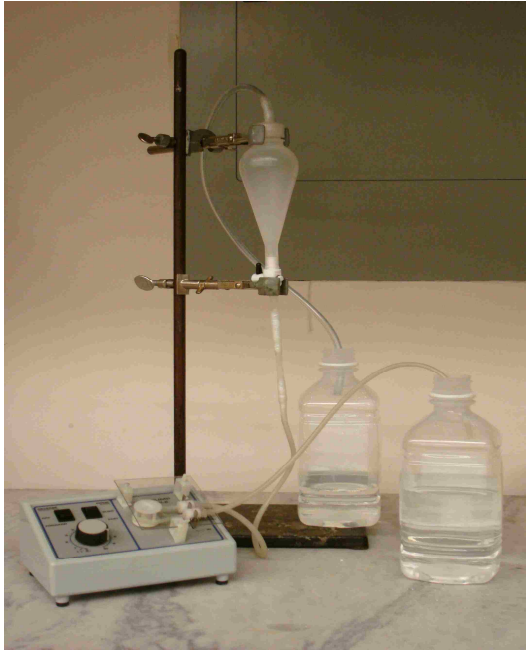
Figure 5.1: A functioning elutriator. Water is drawn from one container and pumped upwards through the funnel, which contains Libby amphibole asbestos fibers. Respirable fibers are eluted out of the top of the funnel, collected in a second container, lyophilized and physically and chemically characterized.
