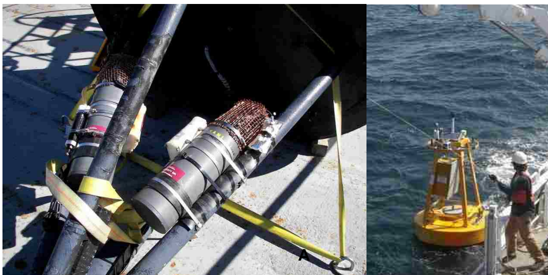
Figure 3.2.1. The SAMI. (A) The SAMI- \text{CO}_2 and the SAMI-pH attached to the spar of the NH-10 buoy, pre-deployment. (B) NH-10 buoy during deployment. The SAMIs are \sim 2 m below the water's surface.
