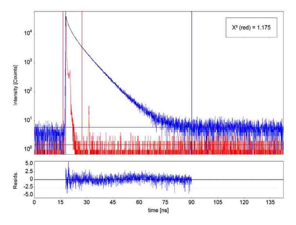
**Figure 5.9:** AcH54I52C37\_AEDANS variant at pH 4.79 in 3 M gdnHCl at 20 °C fitted globally with three exponentials. Data are shown in blue; Instrument response function is shown in red; Black solid line is a triple exponential fit to the data. Residuals below show how well the data fit to a three exponential equation.
