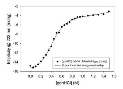
**Figure 2.6** A typical gdnHCl protein denaturation titration monitored at 222 nm using an Applied Photophysics PiStar 180 circular dichroism spectrometer (Gly 4 variant Run #2). Data were collected at 25 °C.
