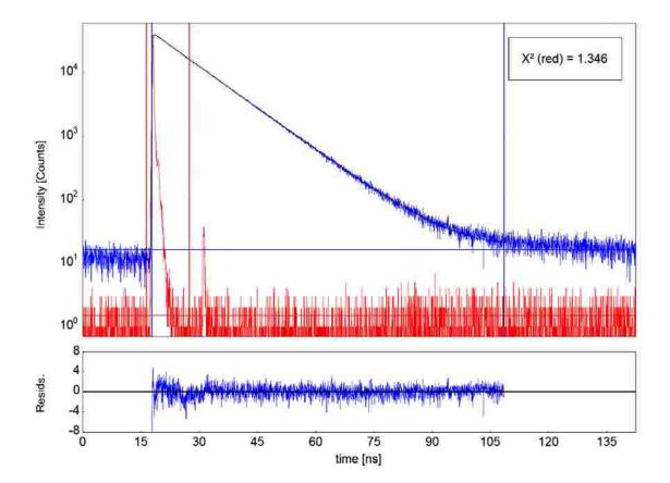
**Figure 5.6:**  $\beta$ -ME-AEDANS used as a control and measured at both pH's 6.36 (shown) and 3.20 for the closed and the opened loop conditions, respectively, in 3 M gdnHCl/3xPi at 20 °C. Probe lifetimes at both pHs were 9.88 ns. Data are shown in blue; Instrument response function is shown in red; Black solid line is a double exponential fit to the data. Residuals below show how well the data fit to a two exponential equation.
