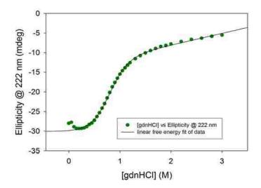
**Figure 3.1:** A typical gdnHCl protein denaturation titration monitored at 222 nm and 25 °C using an Applied Photophysics Chirascan circular dichroism spectrometer for the homopolymeric poly(Ala) variants (NH5A-5 variant Run #1). The solid line is a fit of the data using Eq 3.2.
