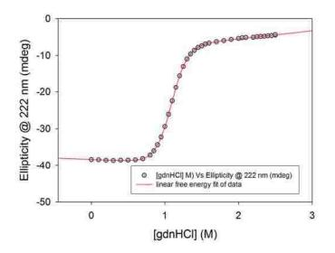
Figure 3.2: A typical gdnHCl protein denaturation titration monitored at 222 nm and 25 °C using an Applied Photophysics Chirascan circular dichroism spectrometer for a cytochrome c' variant (A104H variant Run #2).
