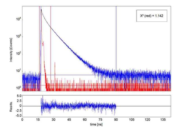
**Figure 5.7:** AcH54I52C37\_AEDANS variant at pH 4.79 in 3 M gdnHCl at 20 °C fitted individually with three exponentials. Residuals indicate an adequate fit of the data. Data are shown in blue; Instrument response function is shown in red; Black solid line is a triple exponential fit to the data. Residuals below show how well the data fit to a three exponential equation.
