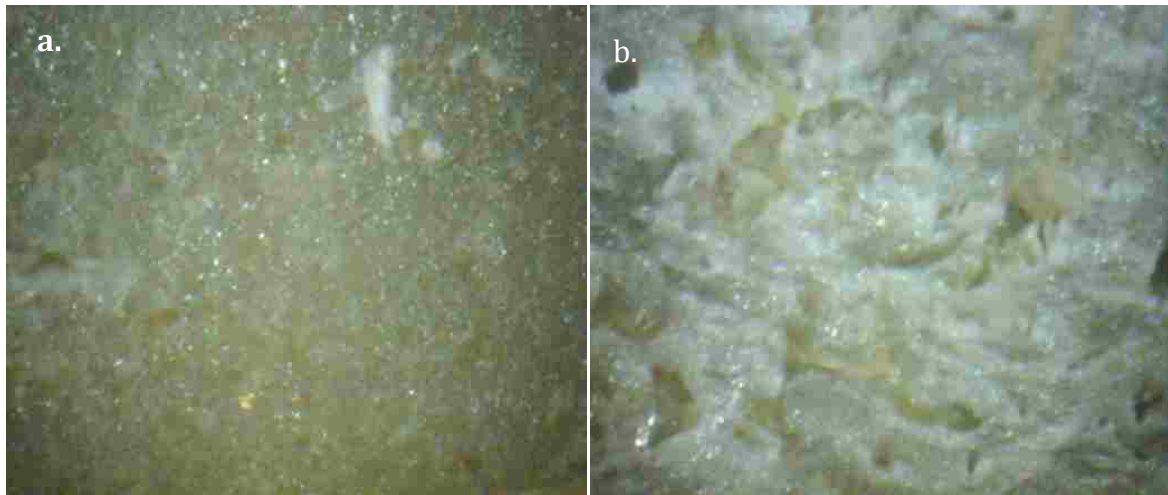
Figure 4.10 Micrographs (400x) of twin-screw compounded WWS sample cross section (a) and tensile fractured surface (b)
