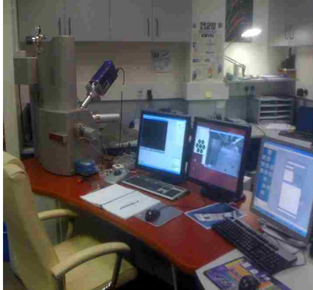
Figure 3.12 The Tescan Mira XMU SEM
