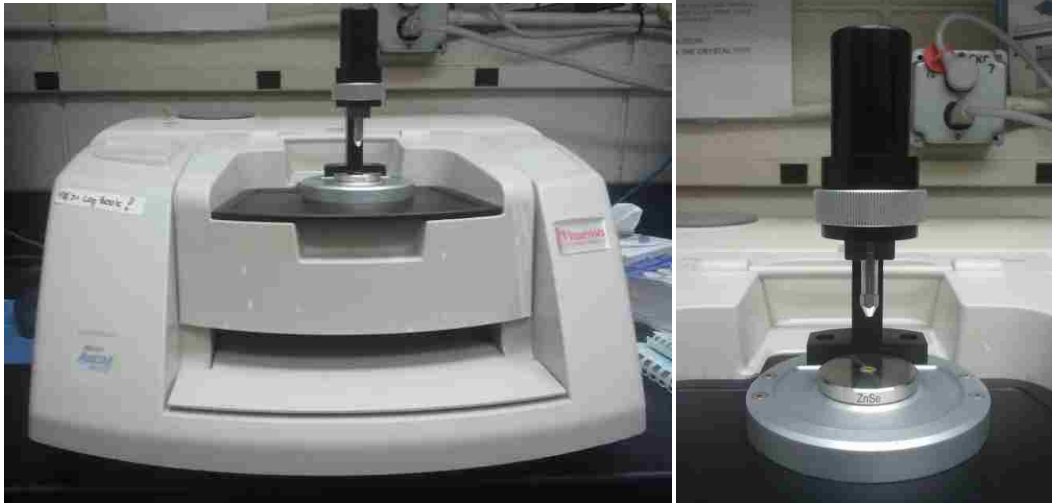
Figure 3.10 The Thermo Nicolet Avatar 370 DTGS FTIR. The entire instrument appears at left, a detailed view of the ATR attachment is on the right
