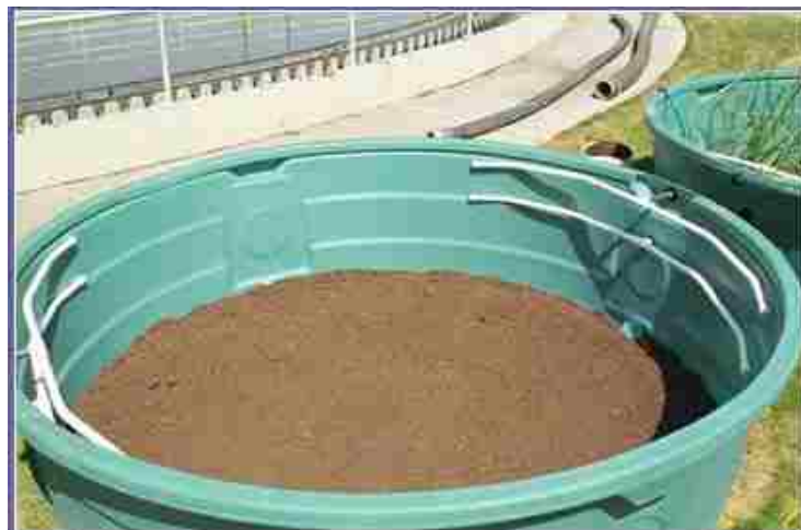
Figure 29. Photo of Cell 2 prior to water and plant introduction. The substrate is Eko-Compost. Note the distribution manifolds for the even distribution of water through the cell.
