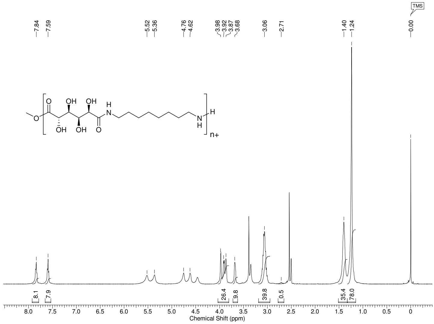
Poly(octamethylene D-glucaramide) post-polymer ^1\text{H} NMR spectrum (DMSO- d_6 ; TMS ref., 0.00 ppm)
