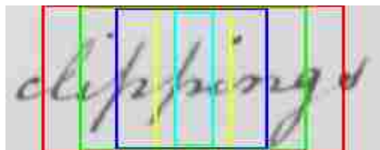
Figure 4.5: This shows a word image with windows of various widths: 200-red, 150-green, 100-blue, 50-yellow, 25-cyan.
