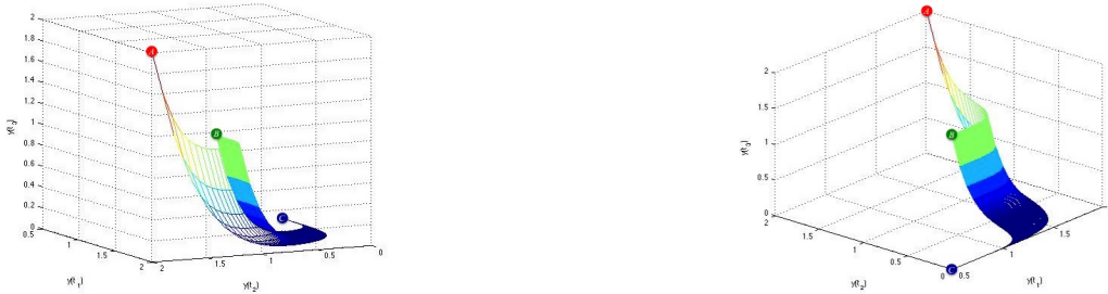
Figure 2.2: This manifold is a mapping f : \mathbb{R}^N \rightarrow \mathbb{R}^M , where N is the number of parameters in the system, and M the number of time points used to characterize the system. These time points are often the time values for which the user has data. The model manifold's shape is independent from the data points used, although, there must be a sufficient number of data points. Each system solution for any value of \theta \in \mathbb{R}^N is represented by an individual point on the model manifold – giving a geometric representation of the entire set of systems.
