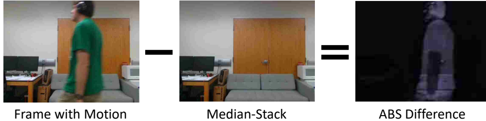
Figure 4.3: Motion removal. We remove frames with motion by taking the absolute difference of each frame with the median-stack image, and removing any frames that violate a threshold. ABS Difference colored here for clarity.
