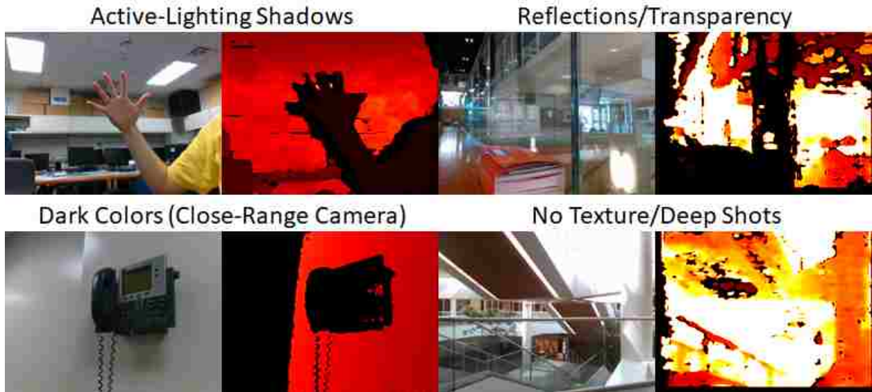
Figure 1.2: Different types of depth-camera noise. Depth cameras exhibit noise differently depending on how they measure distance. In the above examples, each image was captured with an active-lighting/stereo camera. These types of camera tend to struggle with partial occlusions, reflective surfaces, dark colors, and textureless regions.
