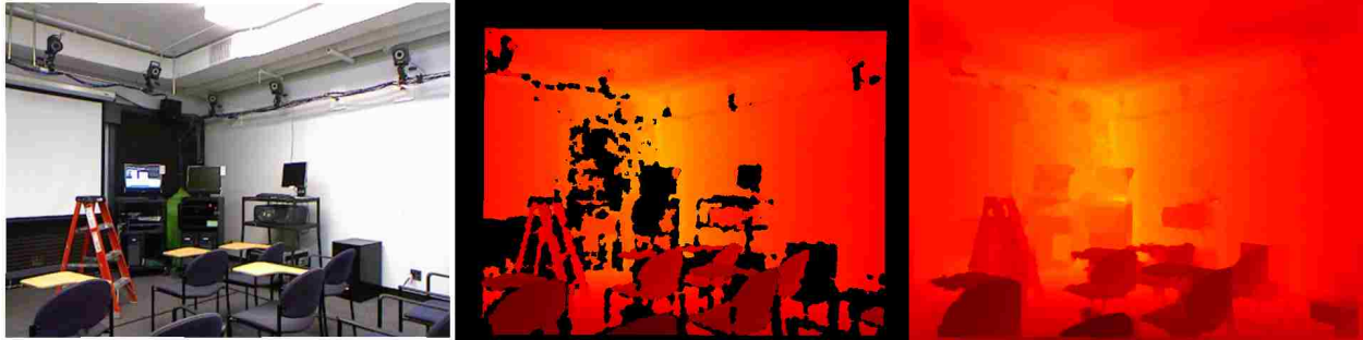
Figure 1.3: Damaged RGB-D image from the NYU Depth V2 dataset compared with its completed ground-truth [30]. There is only one noisy example per clean depth image in this dataset. Left: the original color image. Center: the raw damaged depth map. Right: the hand-corrected ground-truth depth map.
