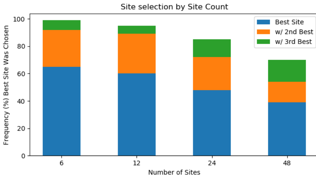
Figure 5.7: Swarm site selection results for different numbers of sites, including second and third best site selection.
