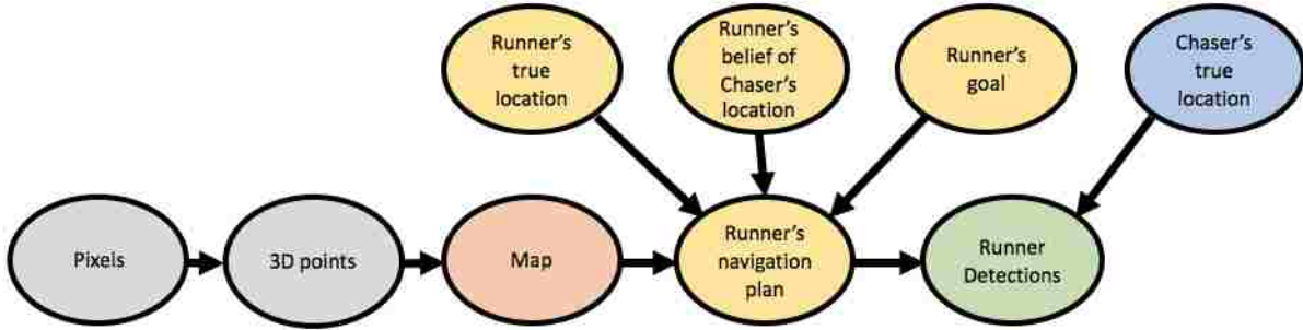
Figure 1.1: Bayesian model of the chaser-runner problem. A map is generated into polygons from pixels. The runner’s plan is determined by the runner’s location, his belief of the chaser’s location, and his goal. Runner detections are based on the runner’s navigation plan and the agent’s true location.
