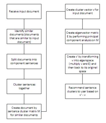
Figure 3.1: This flowchart shows the steps performed in Missing Text Determiner (MTD)
