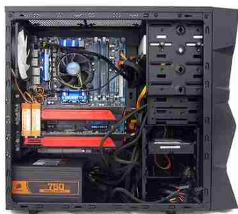
(a) A side view of a personal computer system including a motherboard, graphics card, and power supply connected by physical wires [3]. (b) A three-dimensional X-ray crystal structure of two interacting proteins used to allow yeast cells to adapt to environmental stress [4].
