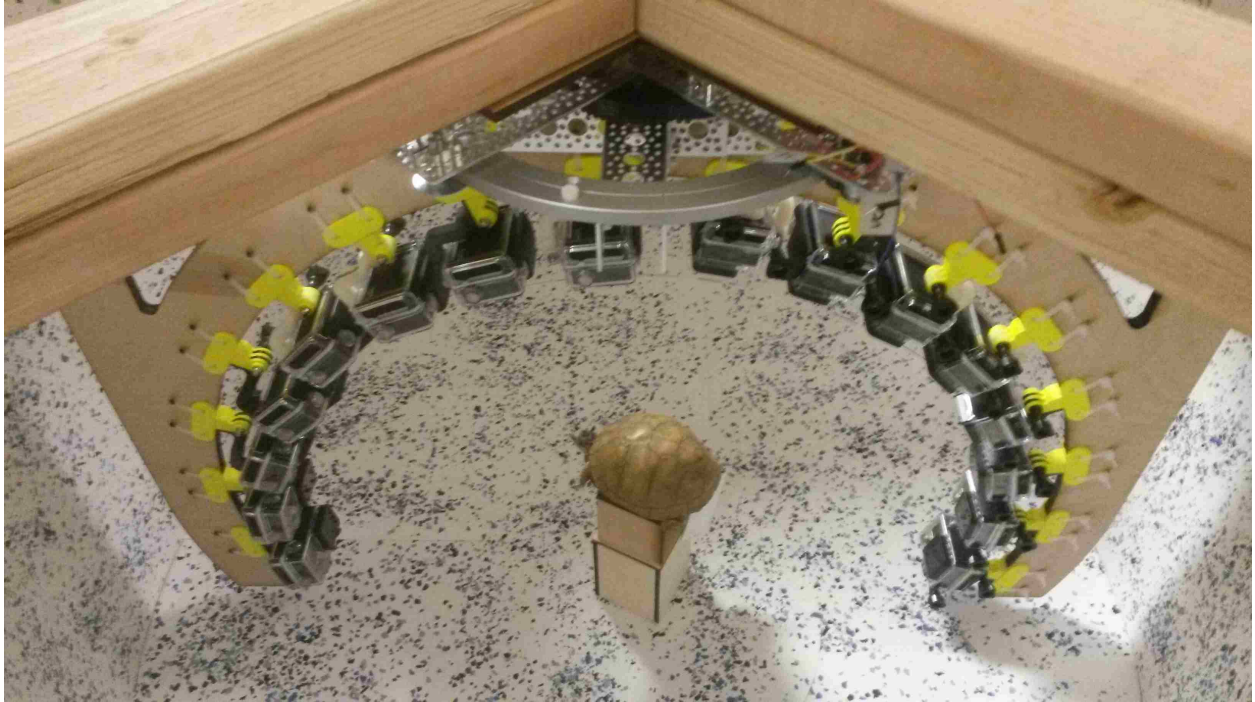
Figure 3.1: Arch containing 16 cameras
