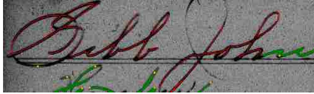
(c) Previously visited pixels are ignored on the second pass. New start points (orange) are the center of the 7 x 7 neighborhood with lowest cost in the unvisited connected components (green).
