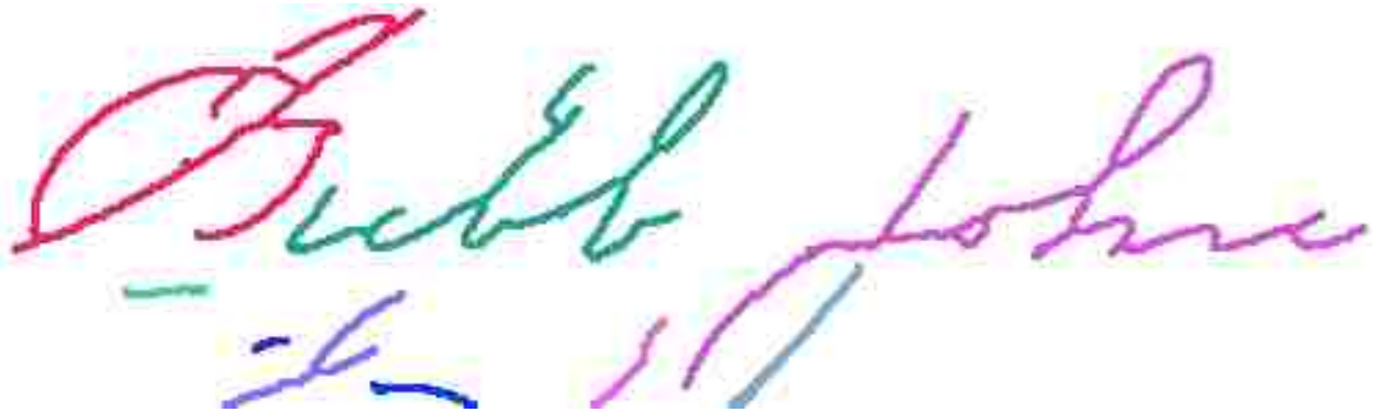
Figure 3.20: Once the strokes are obtained they are joined together into connected components.
