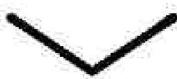
(b) The profile of the distance transform DT is trough-shaped.
