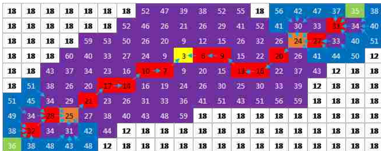
(b) Extending start points in our numerical example. Green pixels (end points) are part of, and complete the (red) optimal path for this image.
